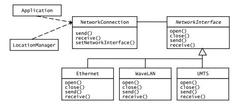
LocationManager configures NetworkConnection with a specific NetworkInterface based on the current location.
